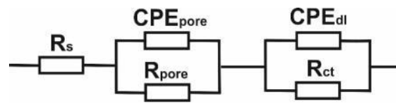
Figure 10. Electric substitute scheme.
