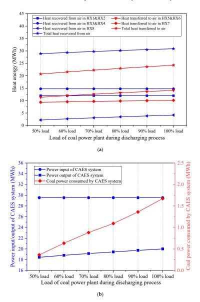
**Figure 14.** Influence of the coal power plant load during the discharging process on the main energy streams of the CAES system, (a) heat energy recovered from and transferred to the air, (b) power streams and coal power consumed by the CAES system.
