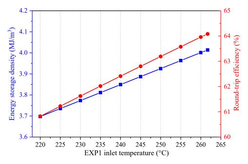
**Figure 11.** Influence of the expander 1 (EXP1) inlet temperature on the performance of the proposed CAES system.
