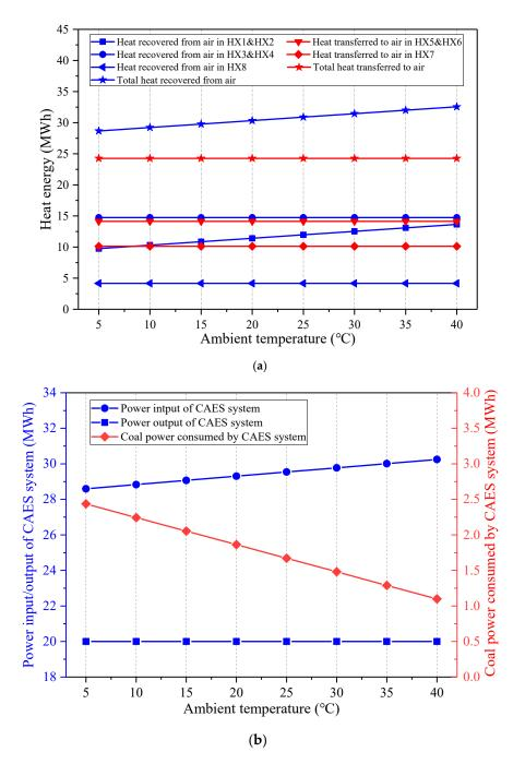
**Figure 6.** Influence of the ambient temperature on the main energy streams of the proposed CAES system, (**a**) heat energy recovered from and transferred to the air, (**b**) power streams and coal power consumed by the CAES system.
