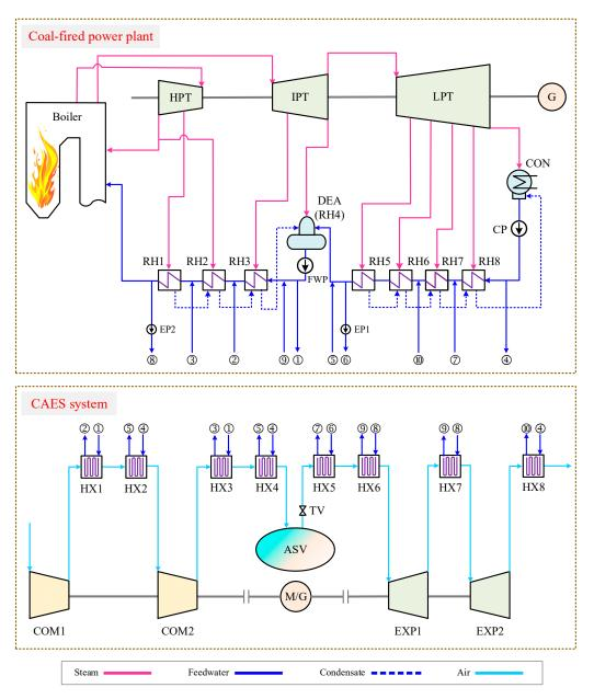
**Figure 1.** Diagram of the proposed compressed air energy storage (CAES) system incorporated with a coal-fired power plant.
