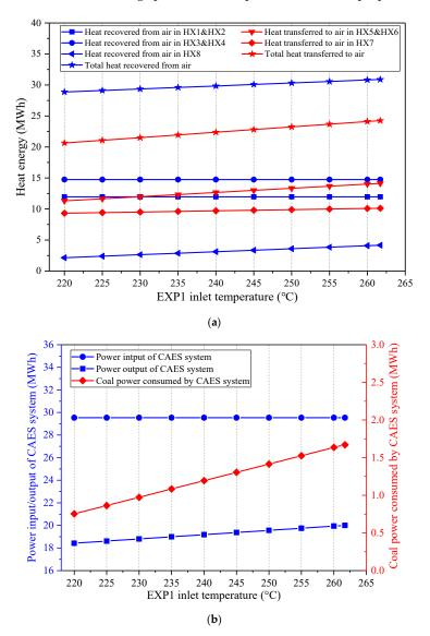
**Figure 10.** Influence of the EXP1 inlet temperature on the main energy streams of the proposed CAES system, (**a**) heat energy recovered from and transferred to the air, (**b**) power streams and coal power consumed by the CAES system.
