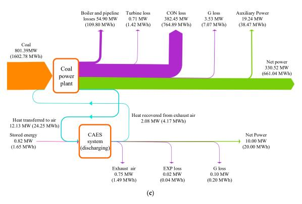
**Figure 4.** Energy flow diagrams of the reference coal power plant and proposed CAES system, (a) reference coal power plant, (b) charging process of the proposed CAES system, (c) discharging process of the proposed CAES system.
