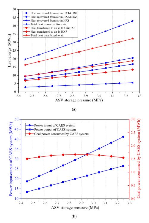
**Figure 8.** Influence of the ASV storage pressure on the main energy streams of the proposed CAES system, (**a**) heat energy recovered from and transferred to the air, (**b**) power streams and coal power consumed by the CAES system.
