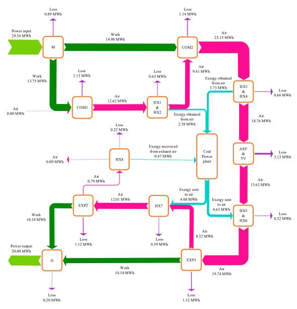
Figure 5. Exergy flow diagram of the proposed CAES system.
