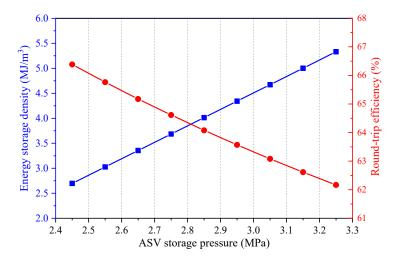
Figure 9. Influence of the ASV storage pressure on the performance of the proposed CAES system.
