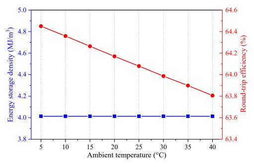
Figure 7. Influence of the ambient temperature on the performance of the proposed CAES system.
