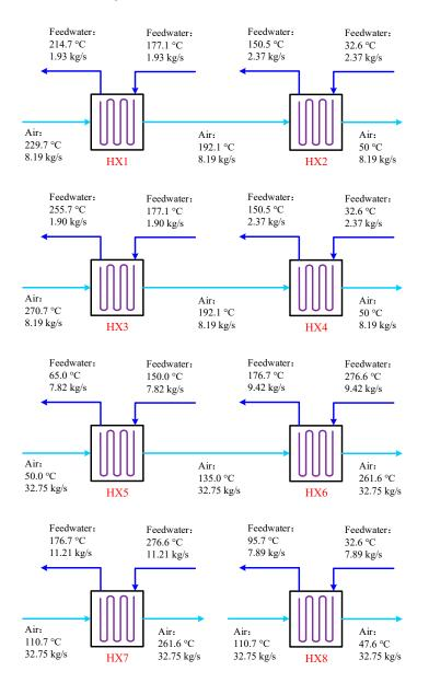
Figure 3. Main parameters of the heat exchanges (HXs) in the proposed CAES system.
