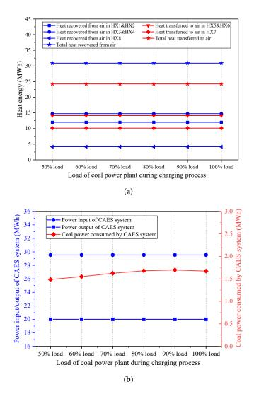
**Figure 12.** Influence of the coal power plant load during the charging process on the main energy streams of the proposed CAES system, (**a**) heat energy recovered from and transferred to the air, (**b**) power streams and coal power consumed by the CAES system.
