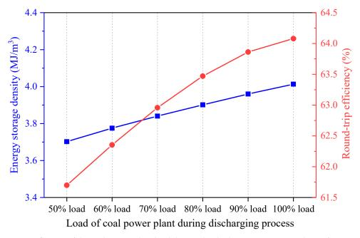
**Figure 15.** Influence of the coal power plant load during the discharging process on the performance of the proposed CAES system.
