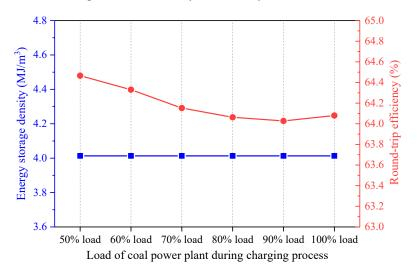
**Figure 13.** Influence of the coal power plant load during the charging process on the performance of the proposed CAES system.
