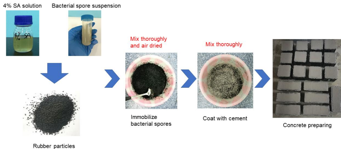
Figure 3. Preparation of self-healing concrete specimens via immobilization of bacterial spores in rubber particles.
