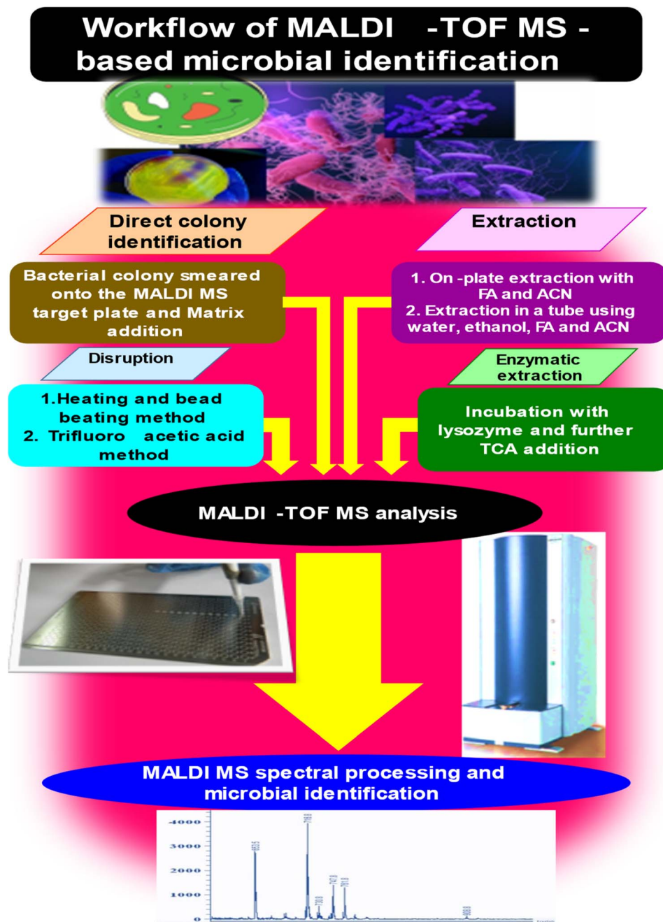
Fig. 2 Overall work flow of steps involved in microbial identification using MALDI-TOF MS. TCA-trichloroacetic acid; FA-formic acid; ACN-acetonitrile.
