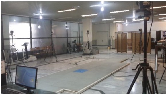
Figure 2. The 7 infrared cameras in Musculoskeletal Research Center.
