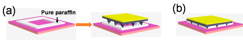
Figure 7. Schematic illustration of the air pressure sensors fabrication, (a) high-purity paraffin was painted on the ITO-PET layer with a closed line frame, and the conductive layer was laminated onto ITO-PET layer; (b) Two layers are sealed through annealing under various vacuum.
