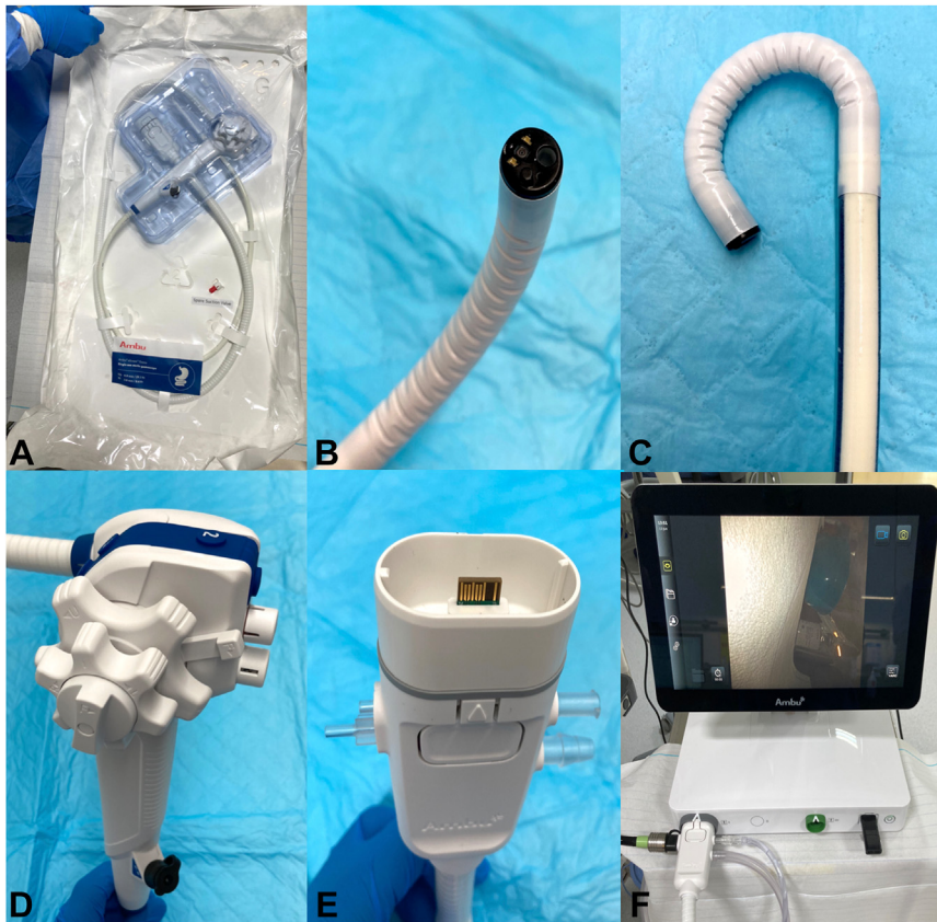
Figure 1. A , The aScope (Ambu, Ballerup, Denmark) is a single-use and sterile endoscope. B , The distal tip has an outer diameter of 9.9 mm, dual LEDs, 140° field of vision, a 2.8-mm working channel, and a water jet. C , Capacity of retroflexion is up to 210°. D , As with conventional endoscopes, there are 2 wheels, 2 locks, and several configurable buttons. E , The scope has a connector that is compatible with standard ancillary devices and tube sets. F , This connector connects to a small processor with light source, and a screen.
