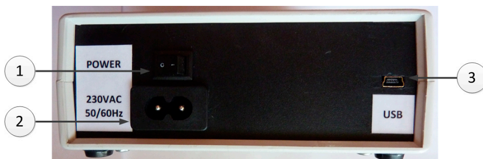
Figure 7. (1) Power switch, (2) alternating current (AC) power connector, and (3) Universal Serial Bus (USB) mini-B connector.
