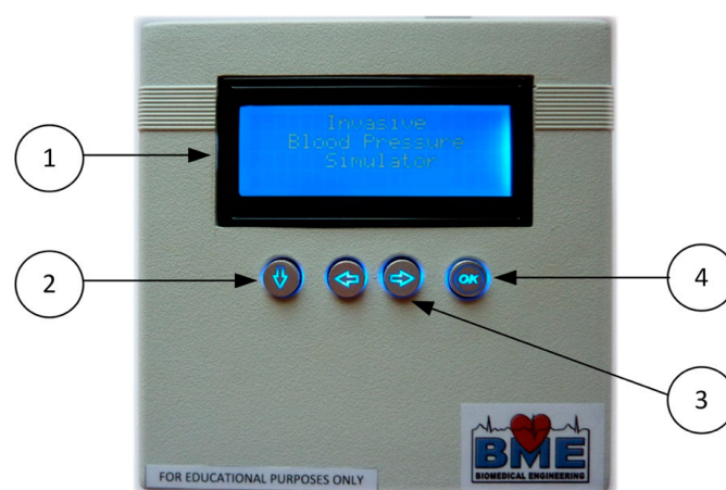
Figure 5. IBPS user interface. On the top are reported (1) an LCD display (2) a navigation button, (3) two setting buttons, and (4) an enter button.
