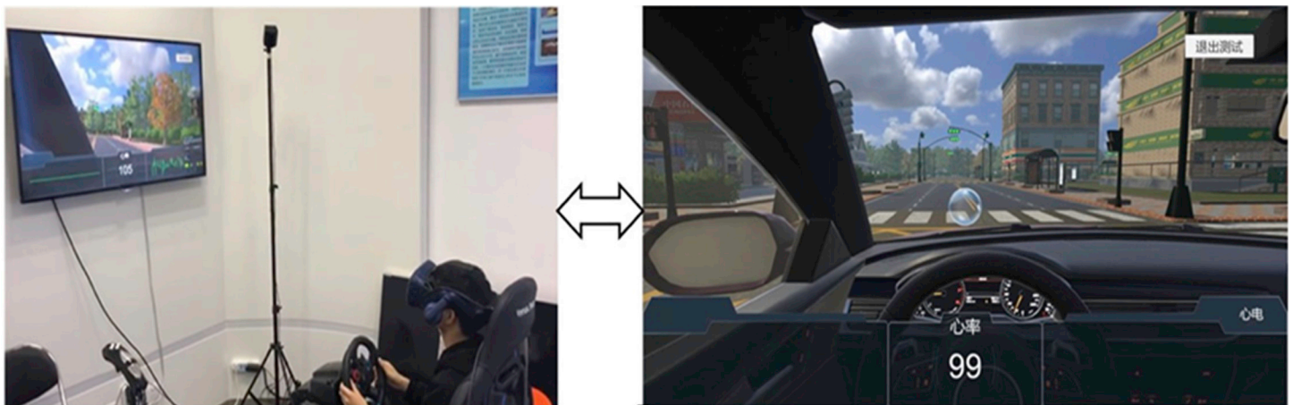
Fig 1. VR driving system. A participant driving in the virtual system (left) and a snapshot containing the ego vehicle, sample of the driving route, intersection, and landmark within the virtual system (right).
