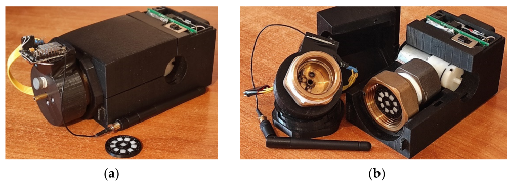
Figure 11. Fluorescence recorder and cartridge used in the experiment: assembled (a) and disassembled (b).
