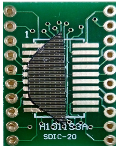
Figure 3. The chip with a set of membranes on the board.
