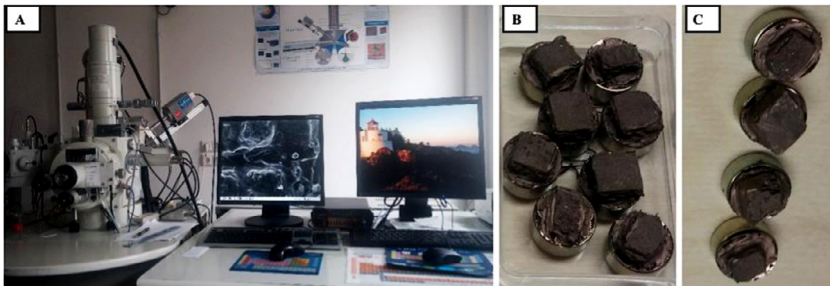
Fig. 6. JOEL JSM 6300 scanning electron microscope, institute for geological sciences and geography at the Martin-Luther University (A). Unreacted (B) and reacted (C) core block samples, cut into 1 cm 3 blocks and mounted on 12 mm by 5 mm aluminium plachets using sticky tabs. They were examined for mineral modifications after the experiments.
