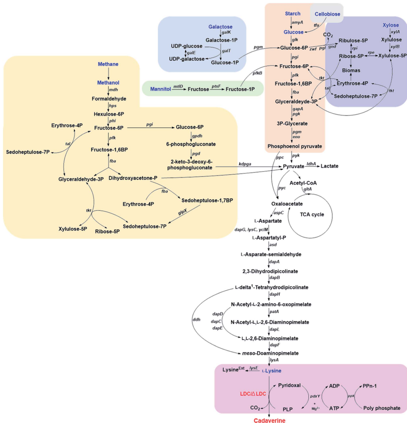
Fig. 2 The pathways for producing cadaverine from glucose, galactose, starch, cellobiose, xylose, methane, mannitol and L-lysine. The following gene abbreviations have been used: gpdh , glucose-6-phosphate dehydrogenase; pgd , 6-phosphogluconate dehydratase, kdpga , 2-keto-3-deoxy-6-phosphogluconate aldolase; ppc , phosphoenolpyruvate carboxylase; pyk , pyruvate kinase; pyc , pyruvate carboxylase; ldhA , lactate dehydrogenase; gltA , citrate synthase; aspC , aspartate aminotransferase; dapG , aspartate kinase I; lysC , aspartate kinase II; yclM , aspartate kinase III; asd , aspartate semialdehyde dehydrogenase; dapA , dihydrodipicolinate synthase; dapB , dihydrodipicolinate reductase; dapH , tetrahydrodipicolinate N -acetyltransferase; patA , acetyl-diaminopimelate aminotransferase; dapL , N -acetyl-diaminopimelate deacetylase; dapF , diaminopimelate epimerase; lysA , meso -diaminopimelate decarboxylase; dapD , tetrahydrodipicolinate succinylase; dapC , succinyl-diaminopimelate aminotransferase; dapE , succinyl-L-diaminopimelate desuccinylase; lysE , lysine exporter; ddh , meso -diaminopimelate dehydrogenase; pdxY , pyridoxal kinase; ppk , polyphosphate kinase; tfu β-glucosidase; glk , glucose kinase; pgi , glucose-6-phosphate isomerase; zwf , glucose-6-phosphate dehydrogenase; pgl , 6-phosphogluconolactonase; tkt , transketolase; tal , transaldolase; xylA , xylose isomerase; xylB , xylulokinase; rpe , ribulose-5-phosphate-3 epimerase; pfk , phosphofructokinase; fba , fructosediphosphate aldolase; mdh , methanol dehydrogenase; hps , 3-hexulose-6-phosphate synthase; phi , 6-phospho-3-hexuloisomerase; fba , fructose-1,6-bisphosphate aldolase; glpX , sedoheptulose-1,7-bisphosphatase; galK , galactokinase; galT , galactose 1-P uridylyltransferase; galE , UDP-galactose 4'-epimerase; pgm , phosphoglucomutase; mtlD , mannitol 2-dehydrogenase; ptsF , fructose-specific phosphotransferase system; pfkB , fructose 1-phosphate kinase; gapA , D-glyceraldehyde-3-phosphate dehydrogenase; pgk , phosphoglycerate kinase; eno , enolase; amyA , α-amylase.
