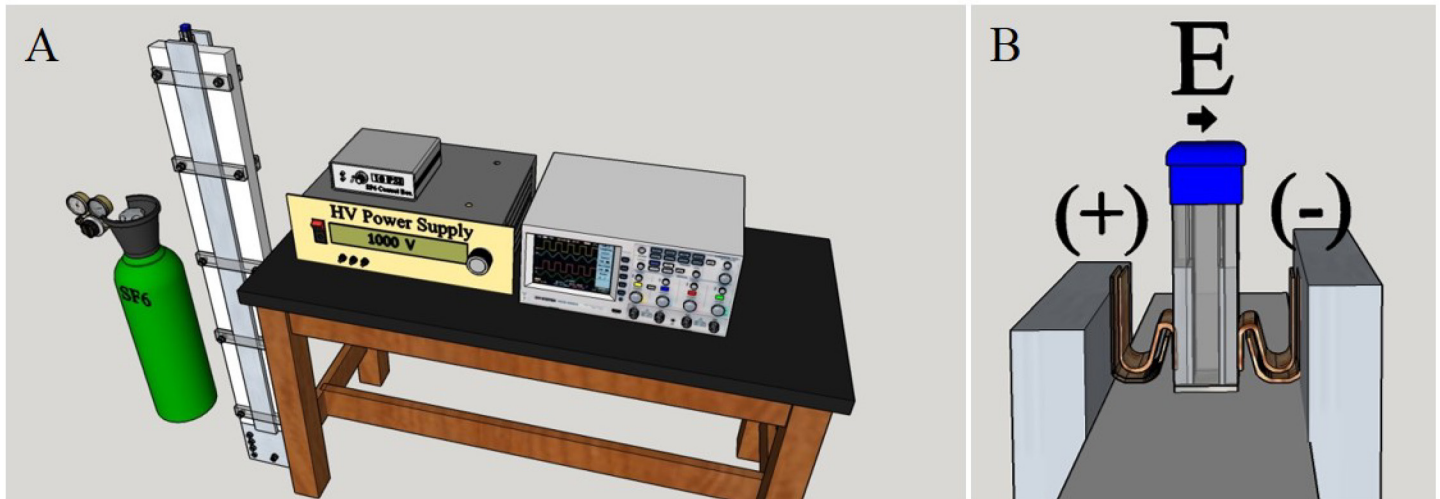
Fig 1. Blumlein line cuvette-based, 10 ns pulser apparatus. A) Drawing of the complete 10-ns set up, including the Tektronix oscilloscope, Glassman high voltage power supply and custom control module for regulating the pressure of SF6 in the spark gap chamber. B) This is an enhanced view of the cuvette and its placement/orientation in regards to the pulser.
