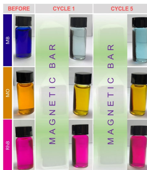
Figure 12. Colors of dyes before photodegradation, after one cycle, and after five cycles.
