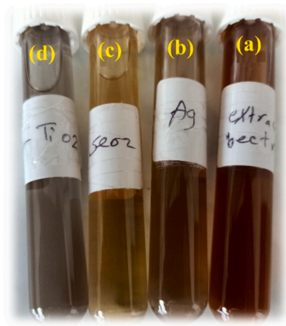
Fig. 1. Color Transformation in Nanomaterial Synthesis: the transformation of a Beta vulgaris L. extract (a) into various nanomaterials: silver nanoparticles (AgNPs, b) and silver-metal oxide nanocomposites (Ag@SeO 2 NC, c; Ag@TiO 2 NC, d).
