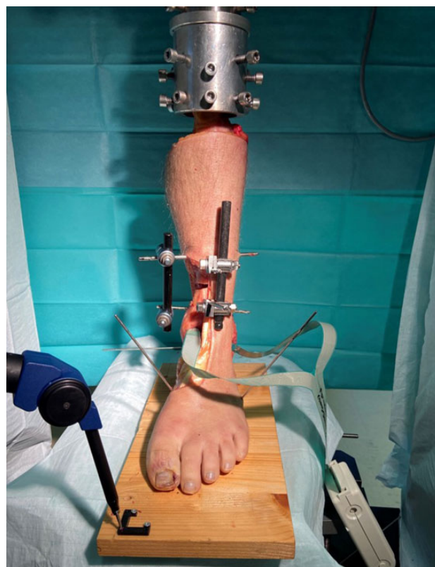
Figure 1. Biomechanical test setup: MicroScribe digitizer (left); Tekscan pressure sensors (right); external fixator device for change of supramalleolar osteotomy.
