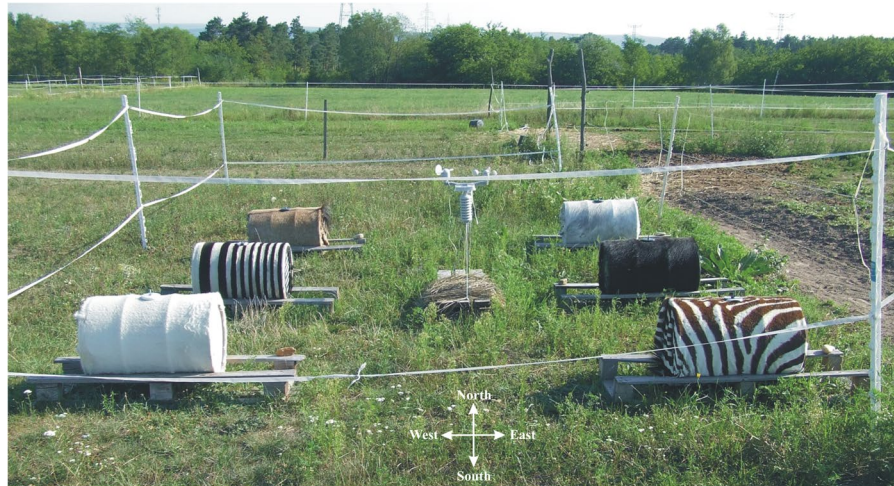
Figure 2. Experimental setup. Arrangement of the six barrels and the meteorological station used in the field experiments. The barrels were laid on a wooden holder which held them at a height of 10 cm above the grassy ground. A circular metal cup covered the hole of the barrel shell and kept the automatic thermometer for measuring the core temperature (photograph taken by Gábor Horváth).
