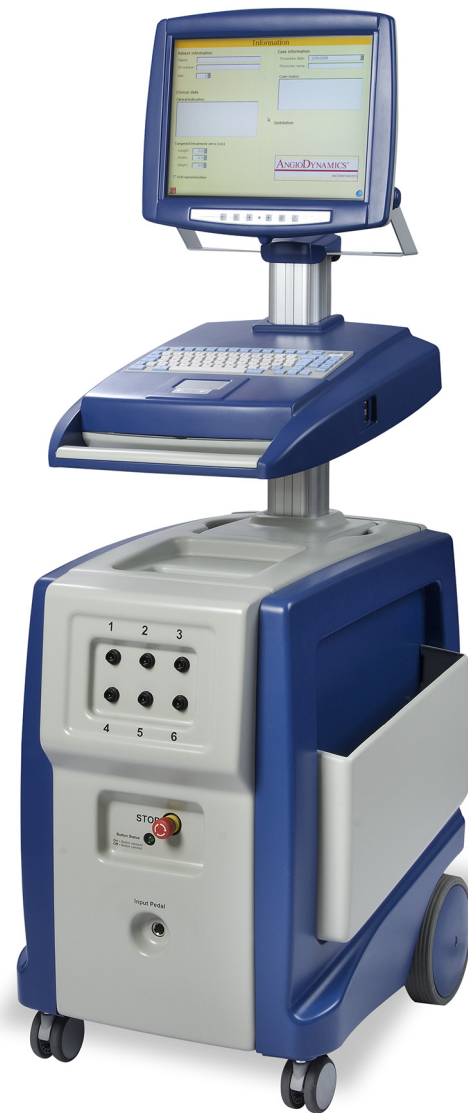
Figure 2 The IRE generator includes an electric power supply, a computer, and 6 output ports that are connected to antennae for the delivery of electric current.
