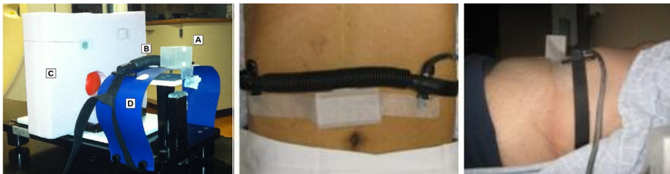
FIG. 2. Experimental setup: Left: (A) infrared marker block tracked with the RPM camera; (B) bellows pneumatic belt; (C) lung-mimicking Styrofoam slab with high-contrast inserts (D) plastic sheet used to mimic the patient surface. Motion platform translates objects in the superior–inferior direction, while the marker block and bellows belt translate anterior–posterior on the corresponding chest wall platform. Middle: Overhead view Patient 9, with the bellows superior to the RPM block. Right: Side view of experimental setup for Patient 4.
