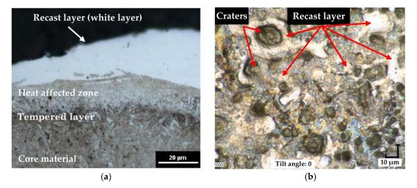
Figure 5. The metallographic structure (a) and surface morphology (b) of 55NiCrMoV7 tool steel.
