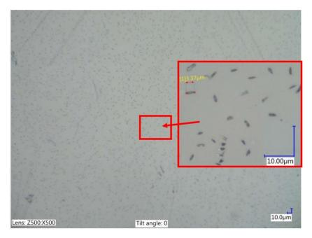
Figure 1. The reduced graphene oxide (RGO) in the dielectric.
