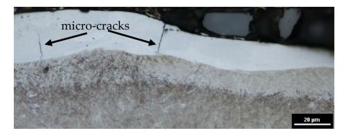
Figure 9. The metallographic structure of 55NiCrMoV7 tool steel after EDM.
