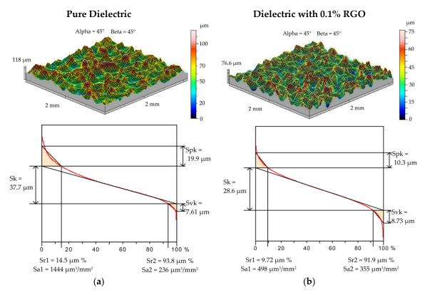
**Figure 3.** The surface texture and Abbott–Firestone curve after electrical discharge machining  $(U_c = 25 \text{ V}, I = 13.5 \text{ A}, t_{on} = 145 \text{ }\mu\text{s})$ : (**a**) pure dielectric and (**b**) dielectric with 0.1% RGO.
