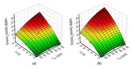
**Figure 16.** The estimated response surface plot for MRR: (**a**) EDM in pure dielectric and (**b**) EDM in dielectric with 0.1% RGO.
