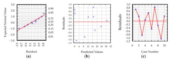
**Figure 14.** Plots of residuals for MRR model, EDM in the dielectric with 0.1% RGO: (**a**) normal plot of residuals, (**b**) residuals versus predicted values, and (**c**) residuals versus case number.
