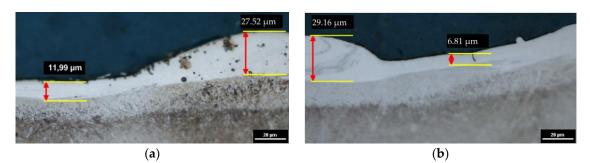
**Figure 8.** Themetallographic structure of 55NiCrMoV7 tool steel after EDM: (**a**,**b**) Uc = 25 V, I = 13.5 A,  $t_{on} = 145 \mu s$ ,  $t_{off} = 50 \mu s$ ; (**a**) pure dielectric and (**b**) dielectric with 0.1% RGO.
