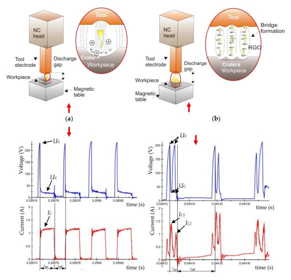
**Figure 4.** The recorded voltage and current waveforms: EDM fluid dielectric. (a) For conventional EDM in discharge time  $t_{on}$ , there is one discharge for the pure dielectric,  $U_0 = 225$  V, U = 25 V, I = 1.2 A,  $t_{on} = 10 \ \mu s$ ,  $t_{off} = 8 \ \mu s$ , and (b) for EDM fluid with 0.1% RGO flakes in the dielectric, in one discharge time  $t_{on}$ , there can be several discharges,  $U_0 = 200$  V,  $U_C = 25$  V, I = 1.5 A,  $t_{on} = 3 \ \mu s$ ,  $t_{off} = 13 \ \mu s$ .
