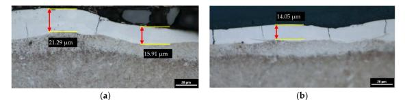
**Figure 7.** The metallographic structure of 55NiCrMoV7 tool steel after EDM; Uc = 25 V, I = 8 A  $t_{on} = 75$  µs,  $t_{off} = 25$  µs: (a) pure dielectric and (b) dielectric with 0.1% RGO.
