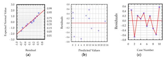
**Figure 13.** Plots of residuals for MRR model, EDM in the pure dielectric: (**a**) normal plot of residuals, (**b**) residuals versus predicted values, and (**c**) residuals versus case number.
