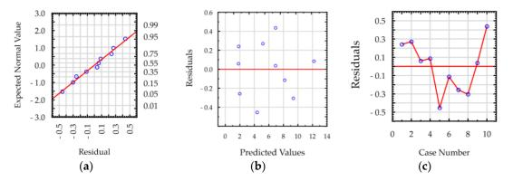
**Figure 11.** Plots of residuals for roughness *Ra* model, EDM in the pure dielectric: (**a**) normal plot of residuals, (**b**) residuals versus predicted values, and (**c**) residuals versus case number.
