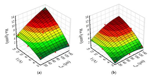
**Figure 15.** The estimated response surface plot for roughness *Ra*: (**a**) EDM in pure dielectric and (**b**) EDM in dielectric with 0.1% RGO.
