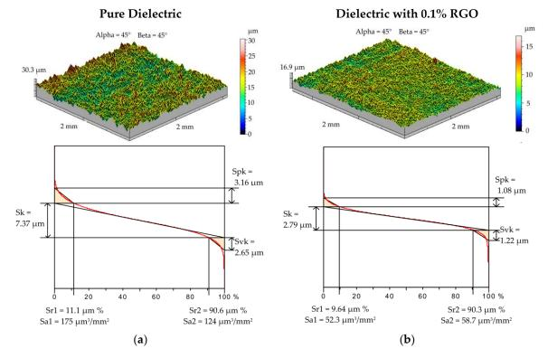
**Figure 2.** The surface texture and Abbott–Firestone curve after electrical discharge machining  $(U_c = 25 \text{ V}, I = 2 \text{ A}, t_{on} = 10 \text{ }\mu\text{s})$ : (a) pure dielectric and (b) dielectric with 0.1% RGO.
