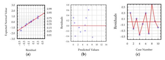
**Figure 12.** Plots of residuals for roughness *Ra* model, EDM in the dielectric with 0.1% RGO: (**a**) normal plot of residuals, (**b**) residuals versus predicted values, and (**c**) residuals versus case number.
