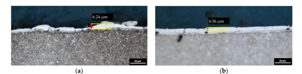
**Figure 6.** The metallographic structure of 55NiCrMoV7 tool steel after EDM; Uc = 25 V, I = 1 A,  $t_{on} = 5$  µs,  $t_{off} = 5$  µs: (a) pure dielectric and (b) dielectric with 0.1% RGO.
