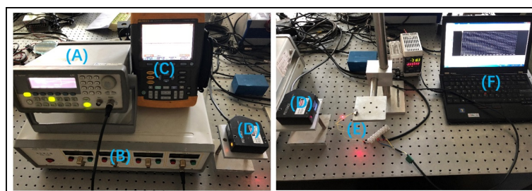
Figure 7. Experimental system: (A) signal generator; (B) amplifier; (C) oscilloscope; (D) laser sensor; and (E) actuator prototype, (F) PC.
