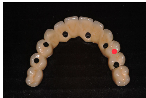
FIGURE 3 Area of the loading procedure. Test performed in the distal fossa on the pontic replacing tooth 24
