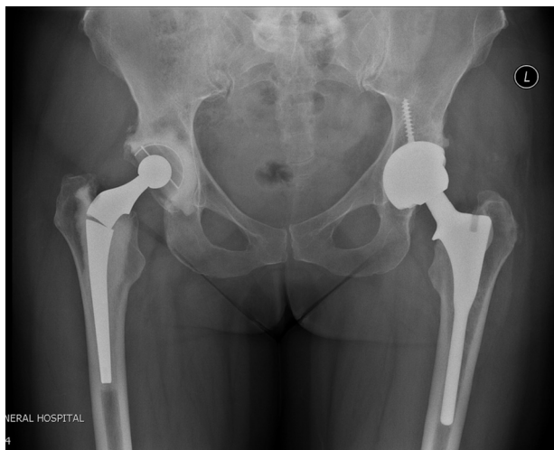
Fig. 1. Case 1. Radiograph shows fracture of right primary Charnley–Elite femoral stem.
