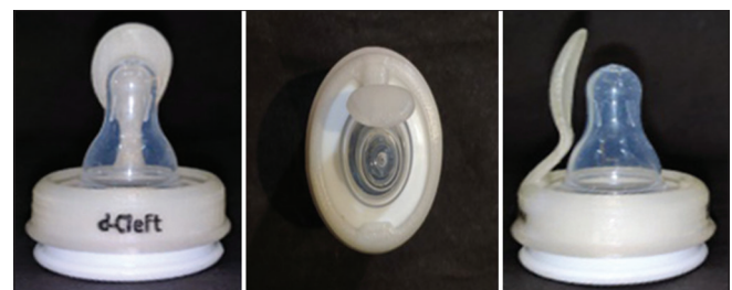
Figure 8: Prototype of the D-cleft made from Flashforge 3D printing machine
