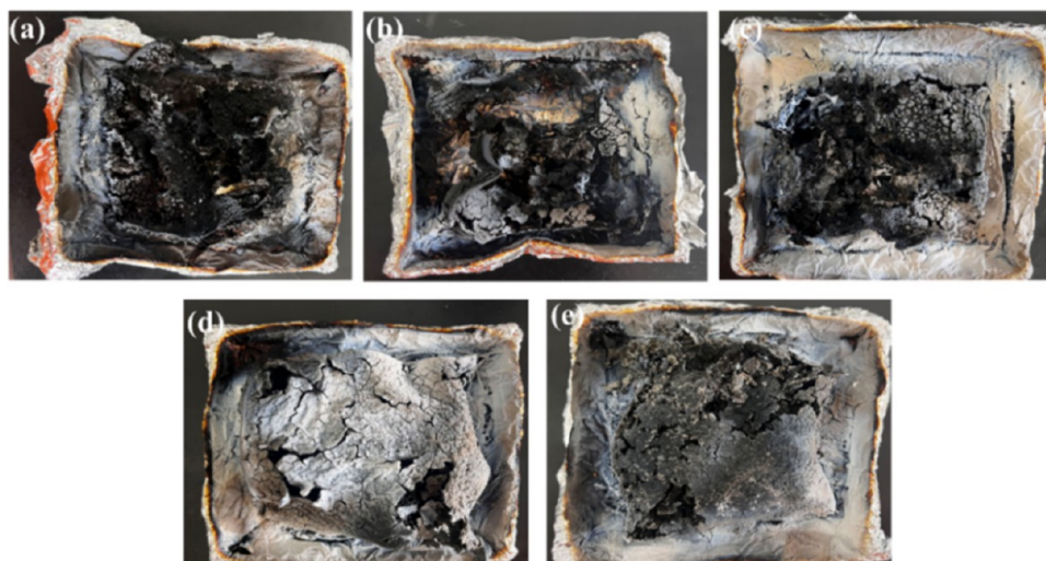
Figure 12. Digital images of char residue for (a) neat RPUF, (b) C/RPUF, (c) N-C/RPUF, (d) A/RPUF, and (e) N-C/A/RPUF.
