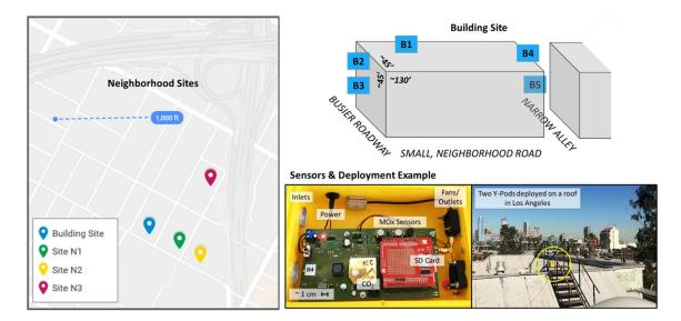
**Figure 1.** The map (**left**) indicates the sampling sites relevant to this paper, the diagram (**top right**) indicates where sensor systems were deployed at the Building Site, and the photos (**bottom right**) show the inside of a Y-Pod and a deployed Y-Pod.
