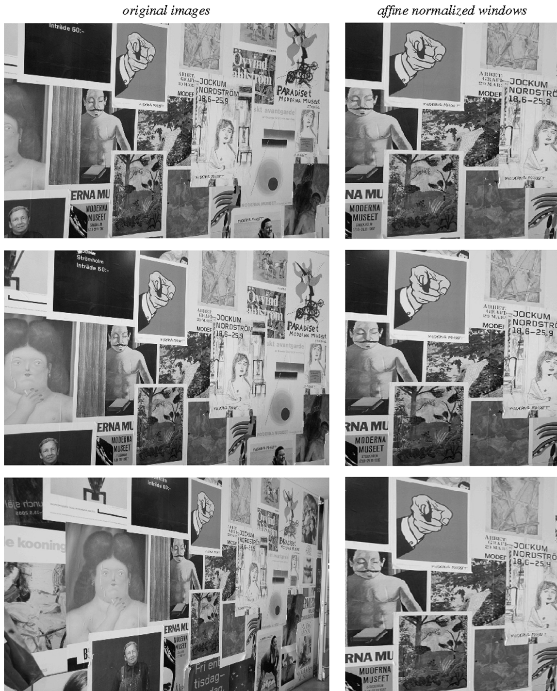
Figure 14. Illustration of how affine invariance can be achieved by normalization to an affine invariant reference frame determined from a second-moment matrix. The left column shows three views of a wall at Moderna Museet in Stockholm with different amount of perspective foreshortening due to variations in the viewing direction relative to the surface normal of the wall. The right column shows the result of performing affine normalization of a window in each image independently (with the windows centered at corresponding image points on the wall) using a series of affine transformations proportional to A = \mu^{1/2} until an affine invariant fixed-point of (81) has been reached. Notice how this leads to a major compensation for the perspective foreshortening effects, which can be used for significantly improving the performance of methods for image matching and object recognition under perspective projection. With regard to receptive fields, the use of an affine family of receptive field profiles makes it possible to define image operations in the image domain that are equivalent to the use of receptive fields based on rotationally symmetric smoothing operations in an affine invariant reference frame. doi:10.1371/journal.pone.0066990.g014
