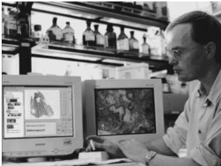
Fig. 6. The remote display station in the pathologists lab consists of 2 monitors displaying the identical information as on the surgery site, the host computer and a joy stick to operate alternatively to the mouse the scanning table.
