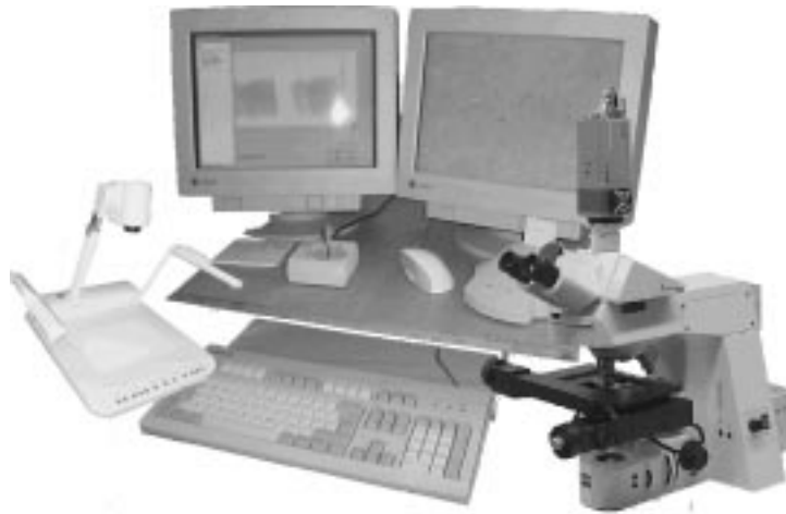
Fig. 5. HSTKOM microscope station with the remotely controllable microscope with scanning table and color TV-camera, the macro device to present the removed tissue before section and to guide the surgery team in frozen section preparation; The host computer; the two monitors display the user interface and the field of view of the microscope; the monitors display identical information as those at the pathology display station and are used also in conference mode.
