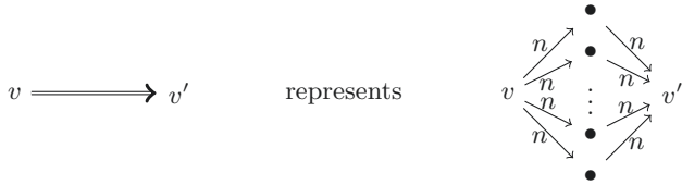
(c) Definition of m -unbreakable link of capacity n with m + 1 intermediate nodes
