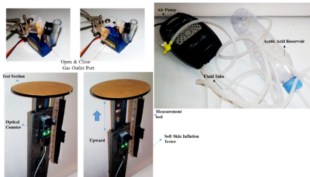
Figure 2. Test equipment including Gas outlet port for depressurizing the swelling soft skin, pump for flowing fluid (acetic acid) through fluid tube and inflation tester for measurement of displacement over time.
