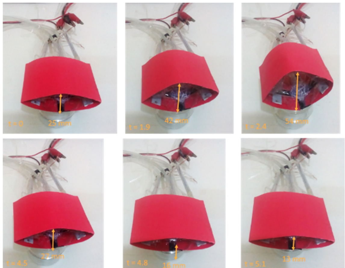
Figure 7. Variation of thickness of small airfoil over time using HEFR technique.
