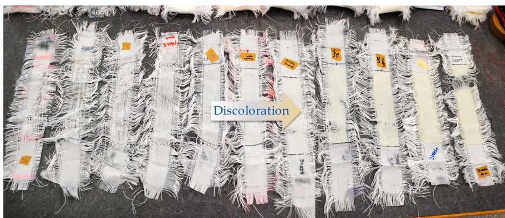
Figure 17. Discoloration, left to right: from 0 to 4684 h, uncoated PET Type II.
