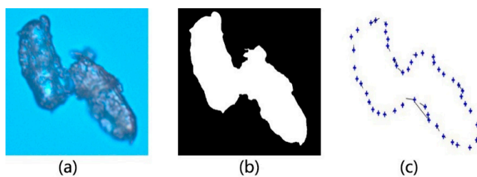
Figure 5. Extraction of Feature points: (a) Original image; (b) Binary image; (c) Feature point.
