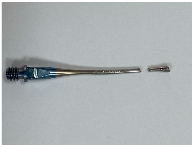
Fig. 1. Picture showing the two parts of the broken phaco tip with multiple pits on its lateral side.
