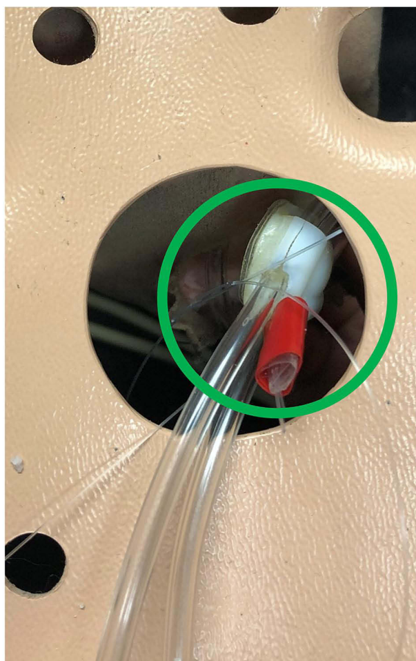
Figure 14 Captured image of successful positioning of the inferior suction base near the apex of the heart, using Introducer Mechanism II.
