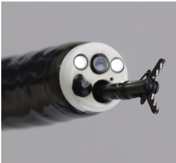
Figure 1. Distal tip of the short-type Clutch Cutter. The blade is 3.5 mm long. The serrated jaw provides accurate targeting (grasping). The outer side of the forceps is insulated so that electrosurgical current energy is concentrated at the blade to avoid burning the surrounding tissue. The forceps is rotatable to the desired orientation.
