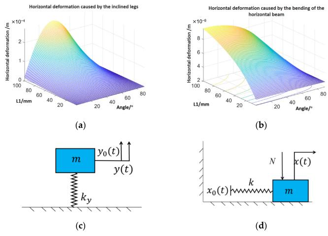
**Figure 2.** (a) The horizontal deformation caused by the inclined legs, (b) the horizontal deformation caused by the bending of the horizontal beam, (c) the vertical dynamic model, (d) the horizontal dynamic model.
