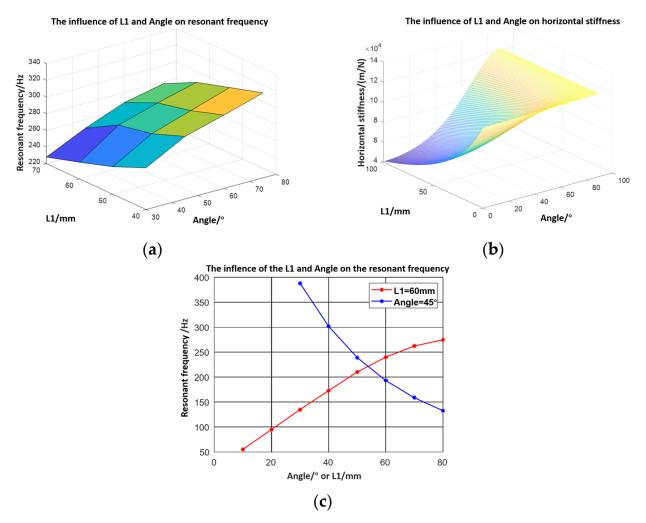
**Figure 10.** (a) Experimental resonance frequency data of robots with varied structure parameters; (b) stiffness of robots with varied structure parameters; (c) influence of L1 and angle on the resonance frequency in simulation.
