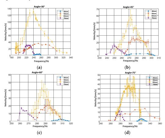
**Figure 6.** (a) Relationship between velocity and leg length when leg angle =  $30^{\circ}$ , (b) relationship between velocity and leg length when leg angle =  $45^{\circ}$ , (c) relationship between velocity and leg length when leg angle =  $60^{\circ}$ , (d) relationship between velocity and leg length when leg angle =  $75^{\circ}$ .
