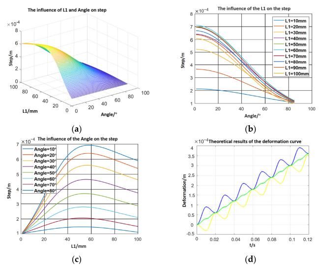
**Figure 3.** (a) The relationship between step, leg length and angle; (b) the relationship between step and leg length; (c) the relationship between step and angle; (d) the relationship between deformation and time.
