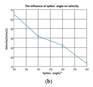
**Figure 4.** (a) The friction factors of different inclined angles; (b) the influence of the inclined angle between microstructures and the horizontal direction.
