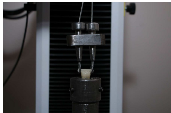
Fig. 4 Custom made double loop made of gear wire hooked around the occlusal bar of the crown
