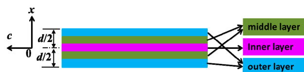
Figure 3. Schematic diagrams positions and different layers in impregnated pressboards.
