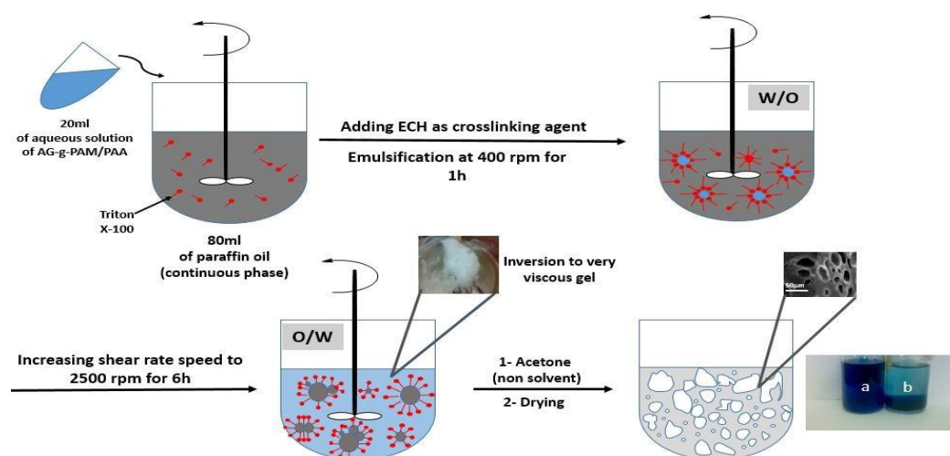
Scheme 3. Schematic representation of crosslinked highly porous grafted gum copolymers preparation whereas the far-left side shows the adsorption of 200 ppm of MB in 100 mL distilled water after 10 min using 0.03 g of (a) crosslinked hydrogel prepared by conventional method (b) crosslinked hydrogel prepared by our method.
