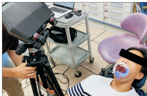
Figure 2. Reference scans for in vivo analysis of trueness. Reference scans of the four spheres are acquired using an industrial-grade scanner (Solutionix C500; Medit Corp., Seoul, Korea) for in vivo analysis of trueness.
