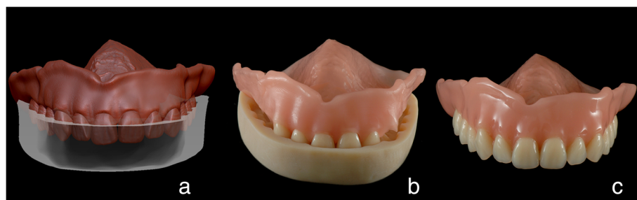
Fig. 3 “The rapid manufacturing (RM) approach” (exemplarily upper denture). a : the virtual design of a transfer key in Zbrush software (Pixologic, Los Angeles, CA, USA) to ensure the proper teeth positioning; b : transfer key put on the denture base and being supported upon the tuber and palatal surfaces; artificial teeth are put into corresponding sockets; c : polished denture with artificial teeth in situ being fixed with cold curing PMMA
