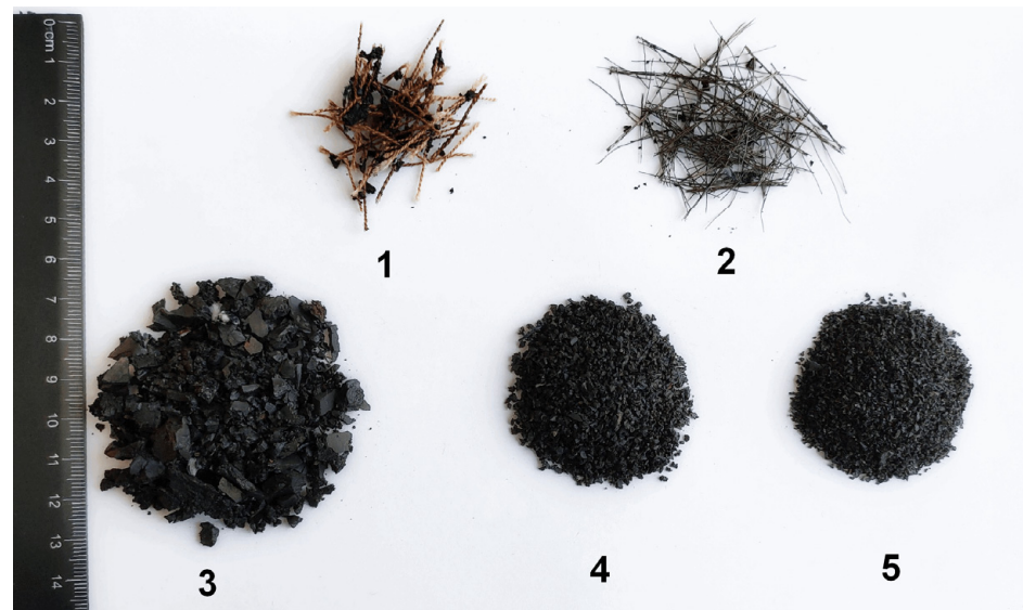
Figure 5. Typical products of cryogrinding. 1—nylon cord, 2—metal cord, 3—large size fraction of rubber crumb (1–5 mm), 4—mean size fraction (1–2 mm), 5—small size fraction (0.1–1 mm).
