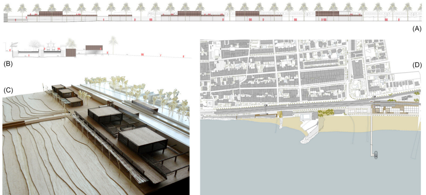
Figure 10. Urban and architectural project for the case study of a stop on the beach of Vilassar-Cabrera (Source: authors' own). (A) General elevation of the maritime façade. (B) Transversal section through the underground passage. (C) Model picture of the prefabricated constructions. (D) General floorplan with different elements used to add order to the maritime seafront: prefabricated buildings, greenway and urban public spaces.
