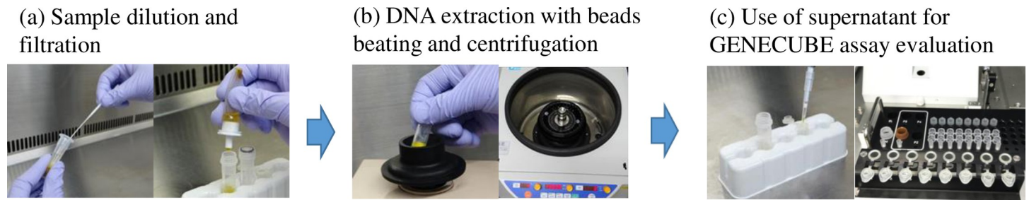
Fig 2. Preparation of test samples for the GENECUBE Clostridioides difficile assay.
