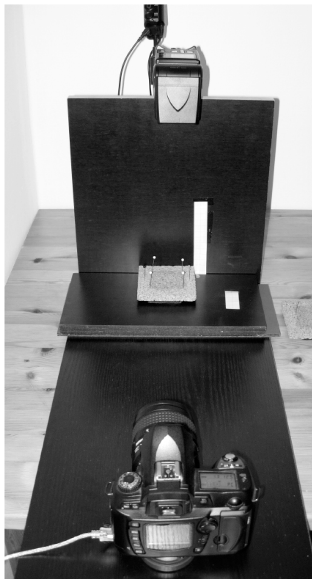
Figure 1 Test arrangement with fixed position of camera and cork plate.
