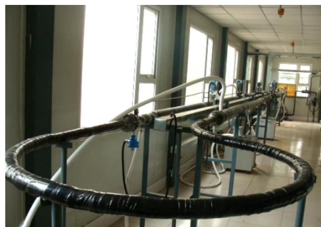
Figure 17. Schematic diagram of the high-pressure hydrate flow loop (a: schematic diagram; b: physical diagram) 51 (photograph courtesy of Shi. Copyright 2021).
