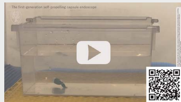
► Video 1 The self-propelling capsule endoscope (SPCE) is controllable in all directions in water (0.00–0.14). Gastrointestinal lumen as observed with the SPCE (0.15–1.02). The SPCE was able to move freely and turn smoothly in the stomach (1.02–2.22).
