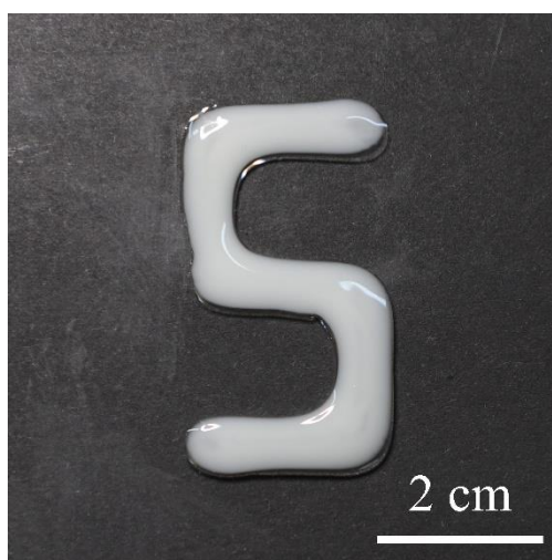
Figure S9. Digital image of a printed PAAm ionogel in "S" shape on PDMS elastomer, related to Figure 2. The molar concentration of AAm is 4 mol L -1 . The ionic liquid is 1-ethyl-3-methylimidazolium ethylsulfate ([C 2 mim][EtSO 4 ]). Before curing, the precursor is transparent. After curing, the ionogel is opaque, presumably due to phase separation caused by the incompatibility between PAAm polymer chains and the ionic liquid.
