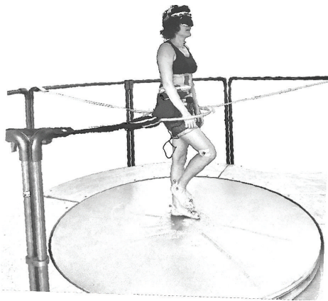
FIGURE 1: Rotating platform. Subjects stepped in place at the center of a platform that rotated counterclockwise at a velocity of 60 deg/s. When the platform stopped, they continued stepping in place blindfolded. In order to prevent subject's translation from the center of the platform, a lightweight hula hoop was fixed to the platform outer railing by elastic straps at pelvic height.
